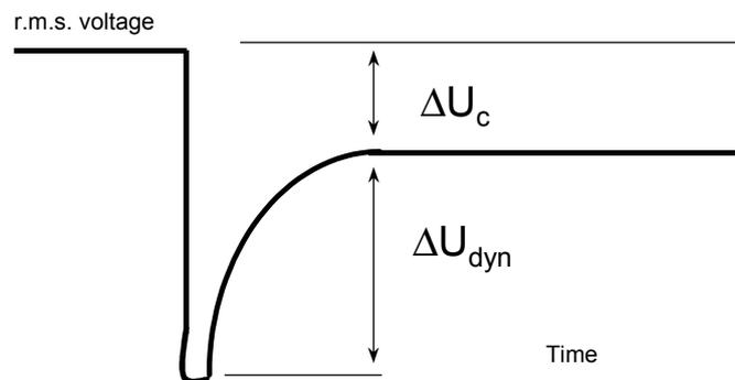
NOTE 1  $\Delta U_c$  is the steady state r.m.s. voltage change, and  $\Delta U_{dyn}$  is the dynamic r.m.s. voltage change.
